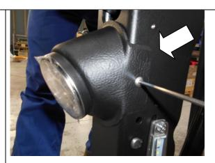
The light support has n.2 holes for fixing to the vertical arm. You must block a side of the support temporarily by proceeding:
