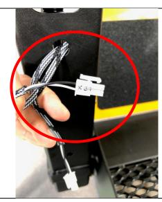
On both the vertical arms of the lift a hole is present where the wiring for the attack of the lights comes out.
