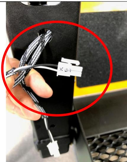
On both the vertical arms of the lift a hole is present where the wiring for the attack of the lights comes out.
