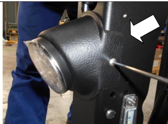
*The light support has n.2 holes for fixing to the vertical arm.
