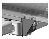
the rear side of the step to the bottom of the vehicle. It is recommended that a sturdy section of the vehicle floor us used. Mount the brackets so that they bridge the gap between step and vehicle floor / chassis. The M8 studs should be placed as vertical as possible. This fixing requires some technical knowledge and own interpretation.
