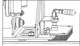
Fix the lock plate(s) with enough spacers at the floor. Adjustment should be made in such a way that the bottom plate slides easily under the lock plate with very little play.
