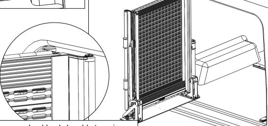
In case the ramp should only be able to swing out, you should position the swing unit in such a way that it stays clear from the door post in the swing out position
