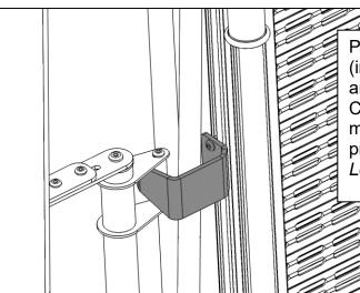
Place the hook at the slit in the first (inner) platform using the M8 bolts and T Nuts.
