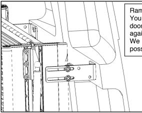
Ramp stop / Ramp Anti rattling device.
