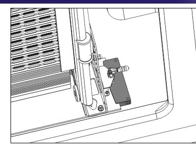
Place the lock plate (red part in picture) in the lock on the bottom plate and close the lock. Make sure the lock plate is aligned with the side of the bottom plate.
