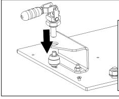
Assemble the lock and the centre piece in the bottom plate assembly.
