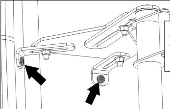
Fix the top bracket to the wall with the two M8 bolts at the rivet nuts that already have been put in place. Fix all bolts firmly
