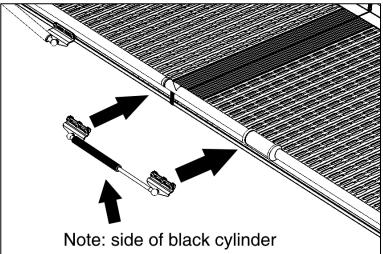
Fix the gas springs to the brackets or mounting plates before installing on the ramp.
