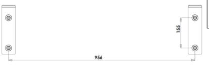
Mark out the position for the 4x M10 mounting bolts for the Mounting plates. Drill the 4 (Ø10.5mm) holes through the floor in a rectangular pattern of 956mm x 155 mm this is a different pattern as for fixed installation
