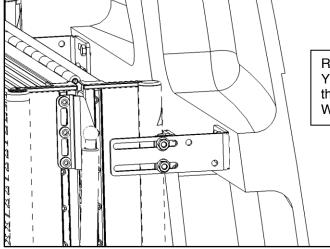
The bracket needs to be fitted with the two rivet nuts M8. (Drill  $\varnothing$ 11 mm holes).
