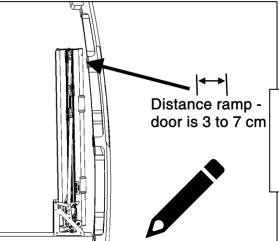
Locate the exact position where the ramp will be fitted at the floor. The ramp should be placed as close as possible to the door, leaving 3-7cm clearance space when the door is closed.
