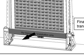
Check if the Feet assembly is standing strait under 90 with the floor. If not tighten or loose the M10 fixations bolts
