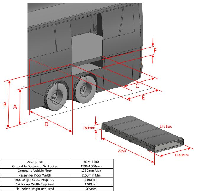
Lift Must be Used with Air Suspension Lowered in Curb Height
