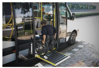
Ramp standard weight: 16Kg (CR Manual) | 36Kg (EPR Automatic)
