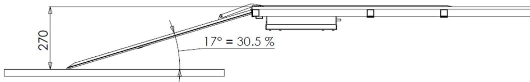
According to the RN 107 the max slope extended or folded out on to a kerb of 150 mm in height, should not exceed 12 %
